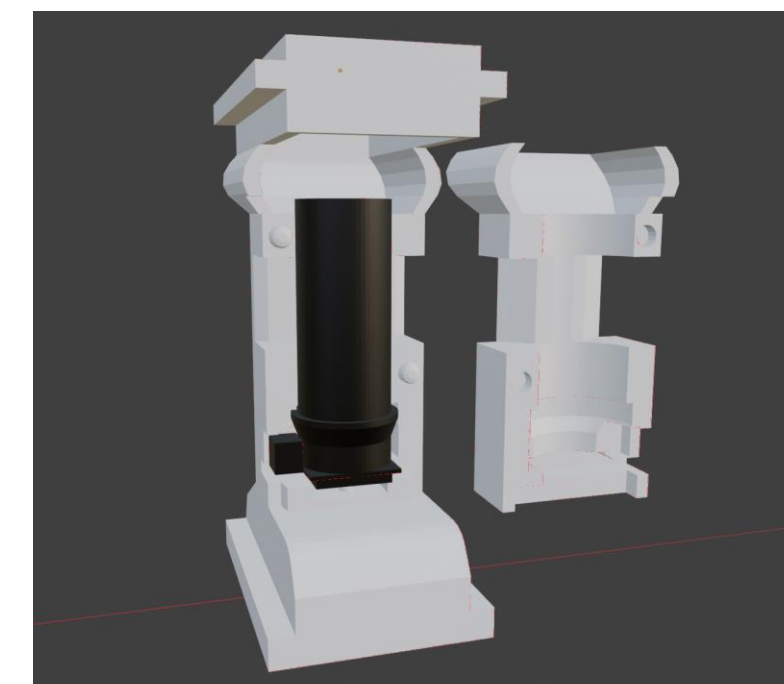
Fig. 4: Microscope Fixture with Light Chamber
